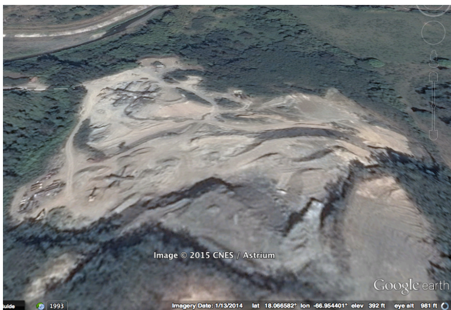
Figure 15. Quarry located on a slope close to the Guanajibo River with few visible runoff controls
